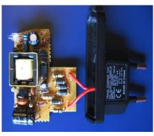
Both PSU's convert Mains AC to DC. The switchmode is cheaper to manufacturer, produces less heat, but can introduce more noise than the Linear Supply. For Best Performance only use a quality Regulated, Isolated Linear power supply.
