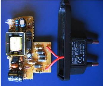
Both PSU's convert Mains AC to DC. The switch-mode is cheaper to manufacturer, produces less heat, but can introduce more noise than the Linear Supply. For Best Performance only use a quality Regulated, Isolated Linear power supply or professional high quality guitar intended switch mode.
