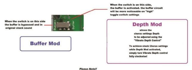
when the Buffer circuit is engaged it will start to induce extra noise when preamp is on its highest settings! Please adjust accordingly to get the least amount of noise!
