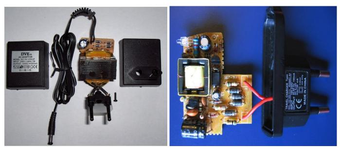
Both PSU's convert Mains AC to DC. The switch-mode is cheaper to manufacturer, produces less heat, but can introduce more noise than the Linear Supply. For Best Performance only use a quality Regulated, Isolated Linear power supply or professional high quality guitar intended switch mode.
